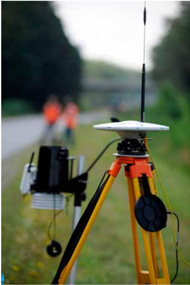
FIG. 3 GPS equipment and weather station at the construction site
