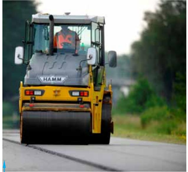
FIG. 4 Roller with GPS Equipment on the roof
