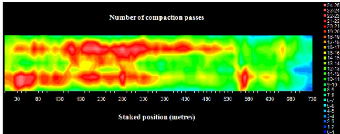
**Figure 4 - Typical Compaction Contour Plot derived from the GPS data**
