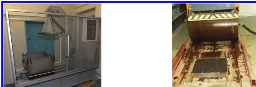
Figure 2. Slab compactor (left) and 2.5 ton roller (right).
