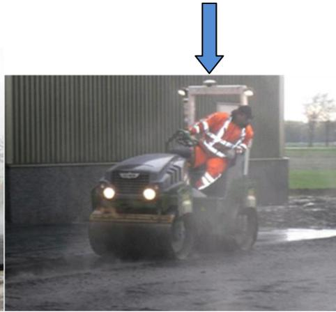
**Figure 5: GPS-equipment on a roller**
