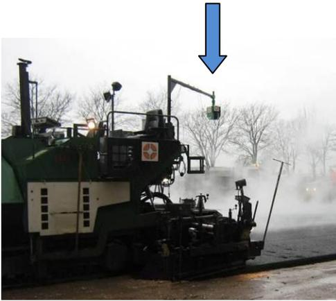
**Figure 4: Laser line scanner on the paver**
