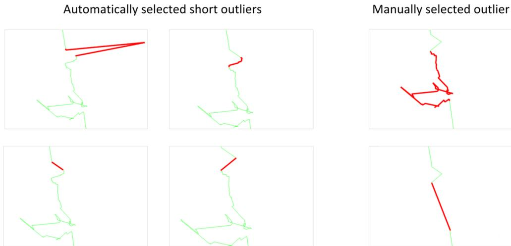
Figure 3. Examples of Identified and Linearized Sections of the Roller's Path
