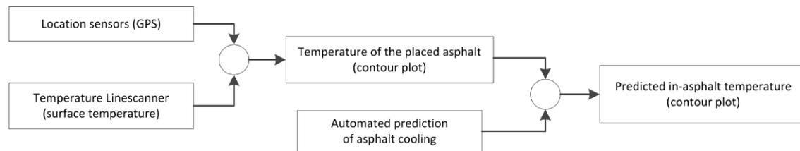
Figure 2. The proposed method to predict in-asphalt temperature
