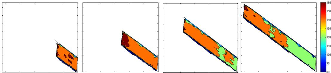
Figure 3. In-asphalt temperature after 4, 8, 12 and 16 minutes after paver started moving.
