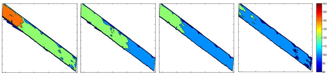
Figure 4. In-asphalt temperature of the paved area after 5, 10, 15 and 20 minutes
