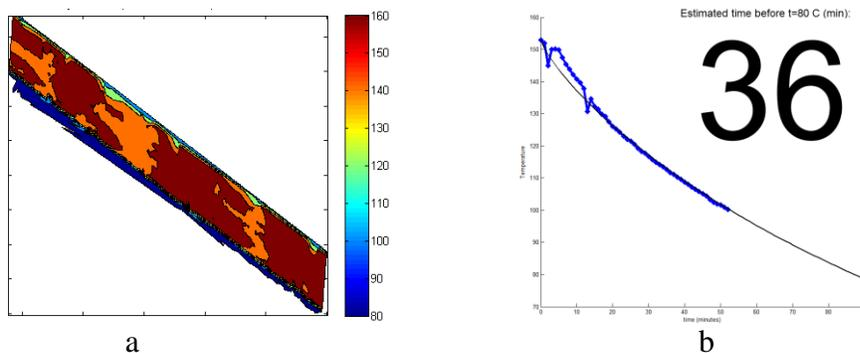
Figure 1: a. Asphalt temperature as measured during laydown;
