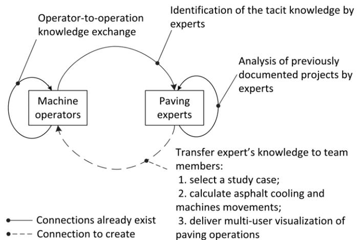
Figure 1. Scheme of the knowledge transfer within the paving domain
