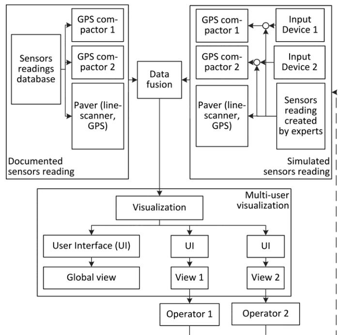
Figure 3. Proposed scheme of the multi-user visualization of asphalt paving operations
