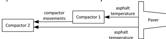
Figure 2. Illustration of the compactor-related information distribution during paving operations
