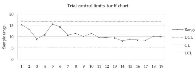
Fig. 3 Trial control limits for the R chart
