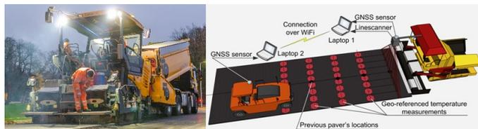
Fig. 1 Laser Linescanner and GPS set up on the paver
