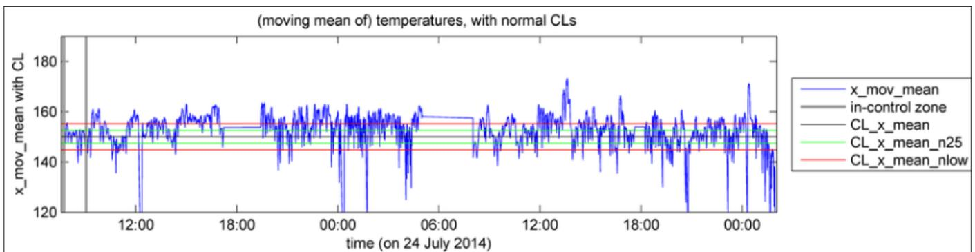
Fig. 8 Moving Average Control chart for a typical asphalt construction project
