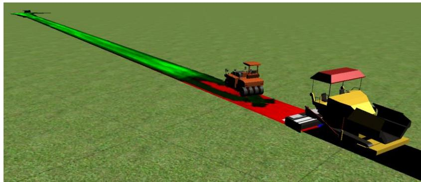
Figure 3. An asphalt paving project reconstructed in PaVE
