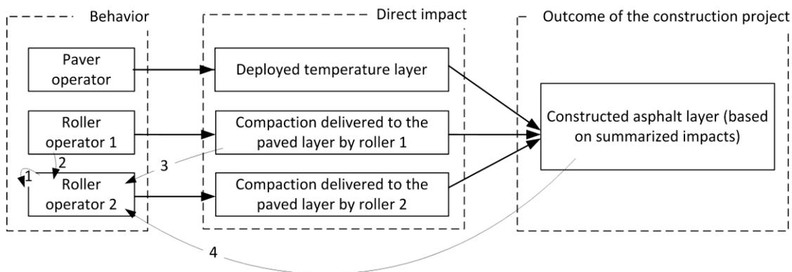
Figure 2. Indicators to describe operational behavior during compaction processes as activities are related to (1) the self-behavior; (2) behavior of other machine operators; (3) direct impact made by the same or other construction machines; and (4) the summarized impact made by two or more machines.
