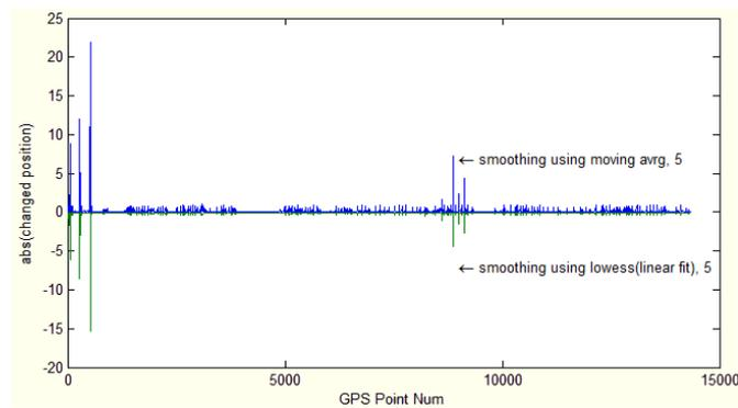
Figure 5: GPS data adjustment using different smoothing techniques
