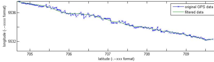
Figure 7: Coordinates of paver received from GPS-receiver and filtered path
