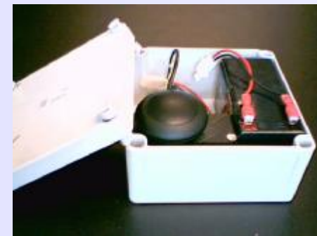
Micodata prototype "off-the-shelf" GPS data loggers (9)
